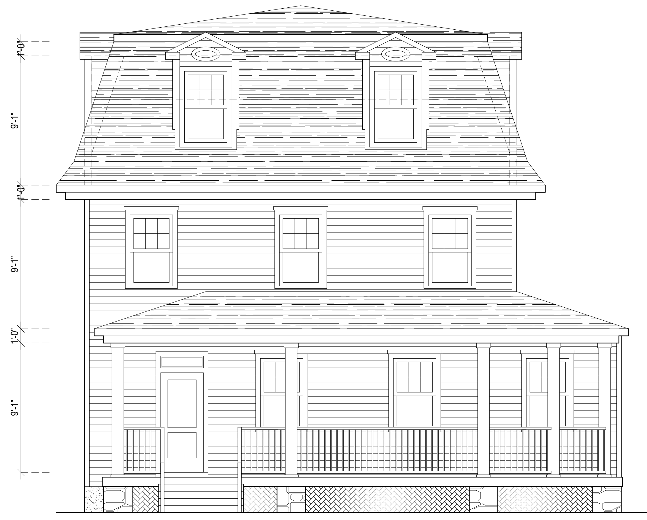
FRONT ELEVATION SCALE: 1/4" = 1'-0"
